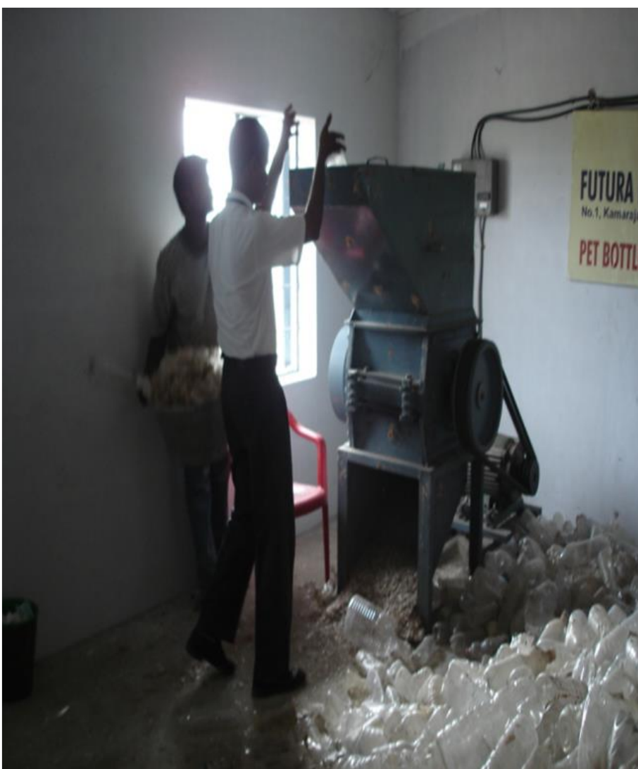
Pet bottles are broken by machine as Chips to reduce its volume
