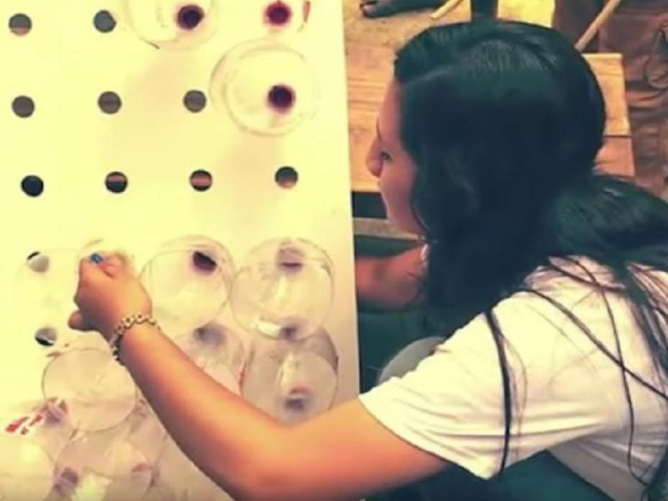
By using recycled plastic bottles and a piece of cardboard covered in equidistant holes, Dhaka managed to create an 'Eco-Cooler' which he says can cool down the summer air. This is because the bottles compress the air in a similar way that your mouth does when pursing your lips.
