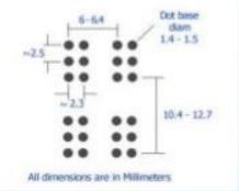
The six dots forming the cell permit sixty three different patterns of dot arrangements.
