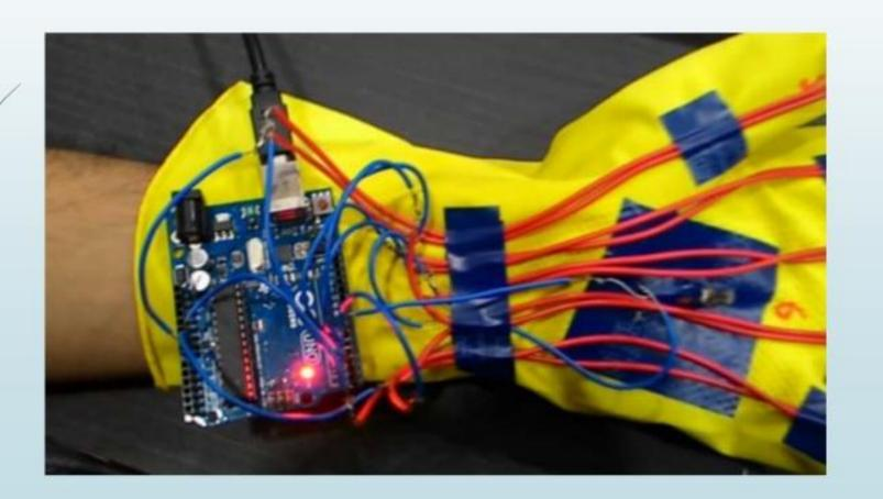
Step 6: The vibratory motors vibrate according to the characters detected following the standard Braille code and the user can identify the characters.
